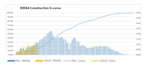
N1064 (X2) construction S-curve shows actual completion progress of 14%, which is according to plan.
