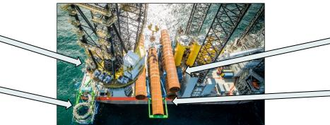
Transportation frame – Holds the monopiles during transfer from port to installation site. Complex steel structure with a 1-1½ year design and fabrication lead-time.
